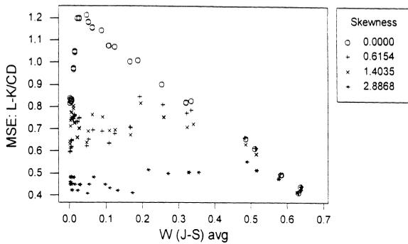
Fig. 3. Relative accuracy of the Lemon–Krutchkoff method vs. classical decomposition: Ratio of MSEs vs.  $W^{J-S}$ .
